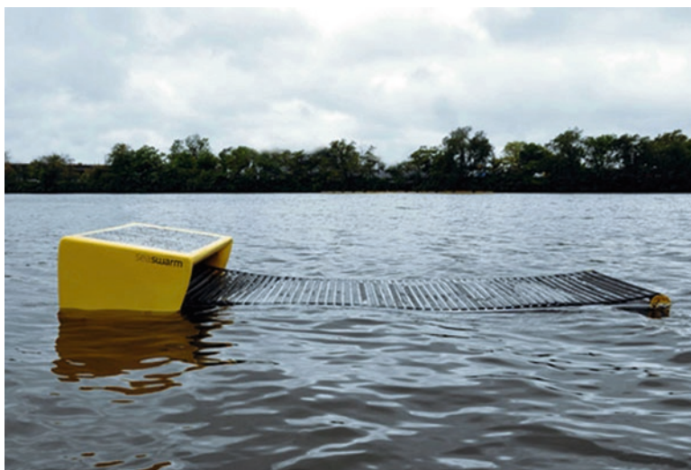
Fig. 14 “Seaswarm” is a nanotechnology-enabled oil-spill-cleaning robot developed by a group of MIT engineers ( TechNews Daily , August 25, 2010). The conveyor belt of the robot is coated with a mesh of superhydrophobic nanowires (Developed by Yuan et al. [73])
