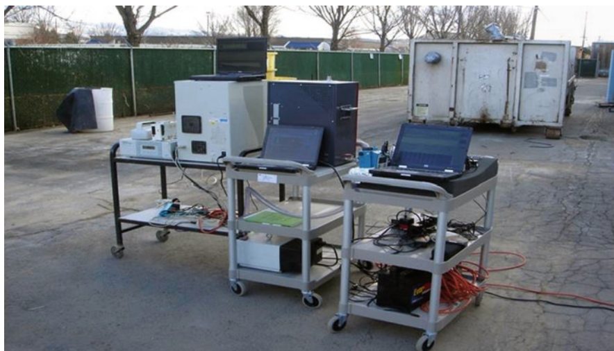
Fig. 8 Example of field application of instruments needed for real-time measurement of number, mass, size distribution, and surface area of engineered nanomaterials (Courtesy of A. Nel)
