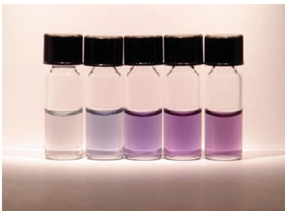
Fig. 9 Following DGU and subsequent fractionation, optically pure SWNT samples are isolated into distinct cuvettes. The color differences between these vials provide clear visual evidence for the success of the DGU process in sorting SWNTs by their physical and electronic structure (Courtesy of Mark Hersam, Northwestern University)
