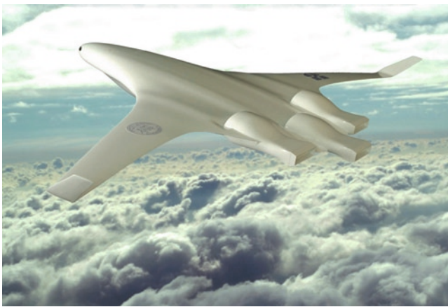
Fig. 11 Nanotechnology will be used extensively in future aircraft designs including this blended wing body subsonic aircraft (Courtesy of Michael Meador, NASA)
