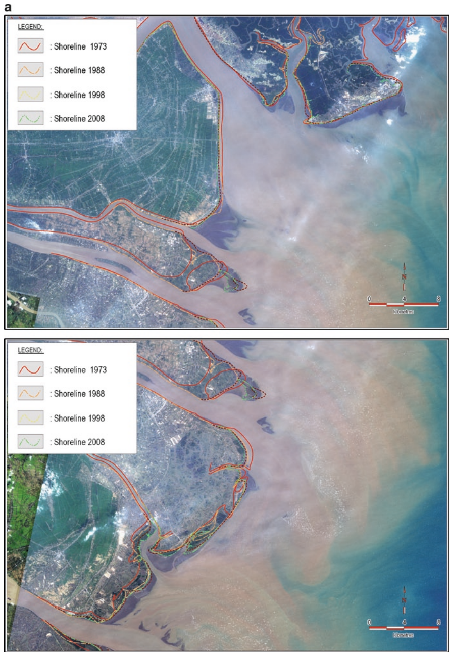
Fig. 18.12 Shoreline change in the Mekong Delta detected from satellite imageries 1973 (red lines), 1988 (orange lines), 1998 (yellow lines), and 2008 (green lines)
