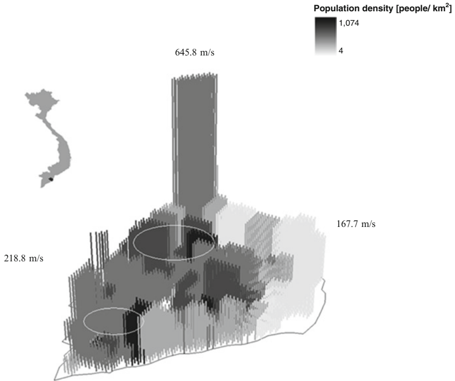
Fig. 21.9 Net wind resources (wind velocity available minus velocity demanded to supply water production over 17.3 km 2 ) in Tra Vinh
