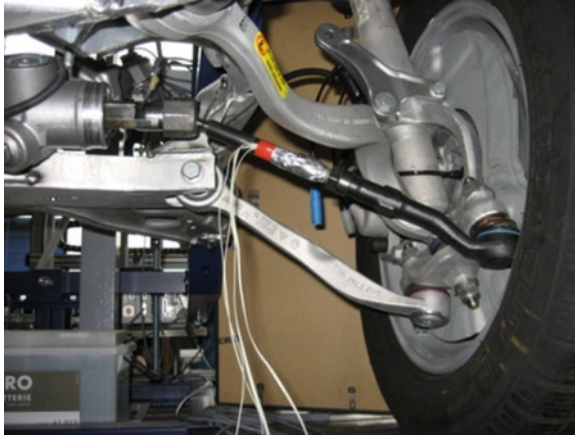
Fig. 44.2 Steering track rod with DMS applied
