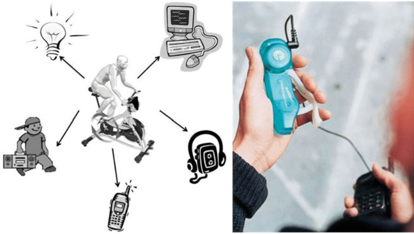
Fig. 1.4 Power recovery from pedaling activity [58] and the Aladdinpower ® charger
