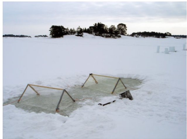
Fig. 9.11 Set-up of an UVA experiment on Baltic Sea ice. One of the tent-shaped frames is covered with UVA opaque foil (PAR treatment) and the other is covered with UVA transmitting foil (PAR + UVA treatment). Photo: © Jari Uusikivi
