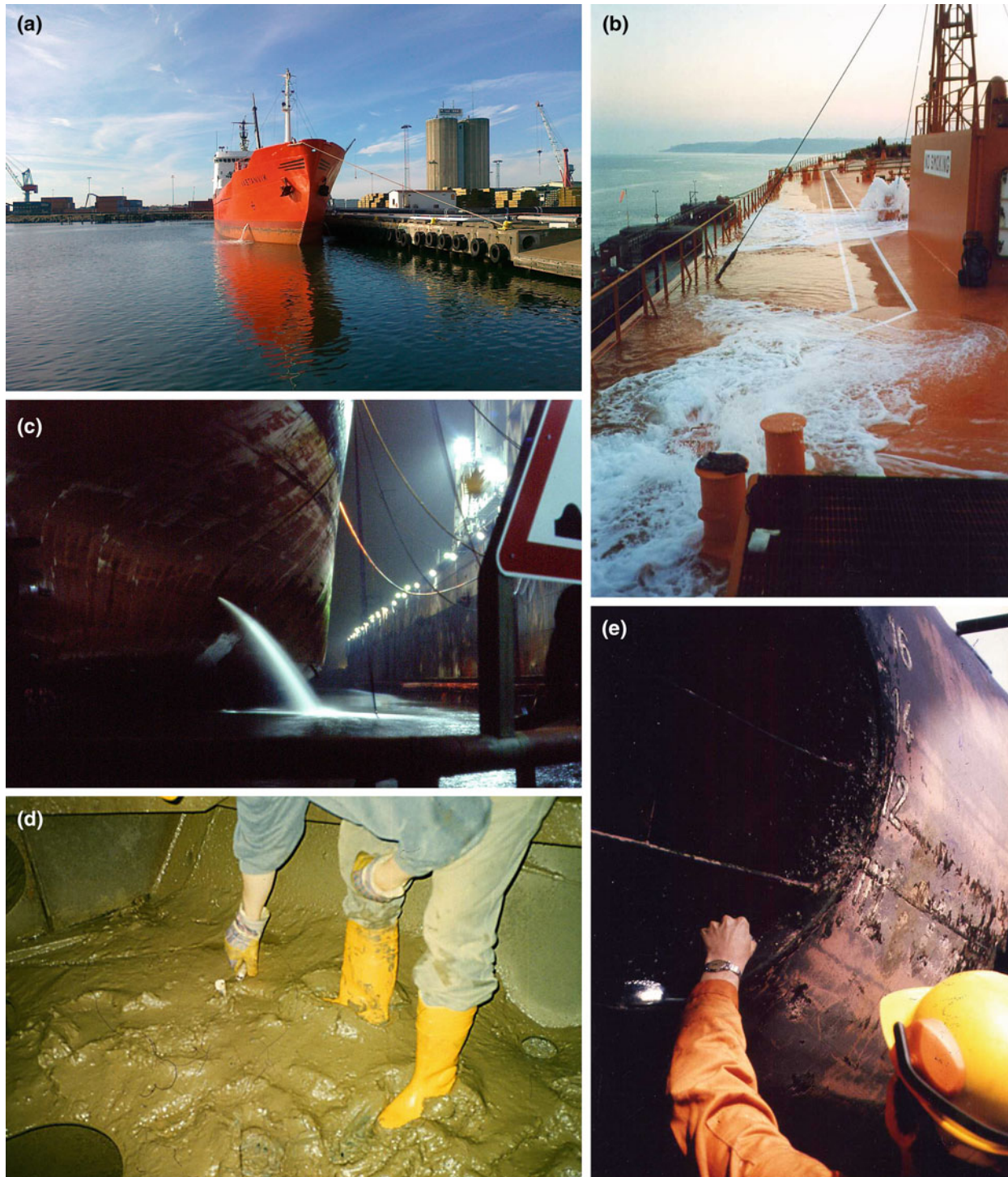
Fig. 5.9 Examples of the shipping pathway of non-indigenous species. (a) Ballast water release in a harbour. (b) Ballast water overflow on deck. (c) Ballast water release in a dock at night. (d) Sediment in a ballast water tank after release of the water. (e) Collection of organisms from a ship's hull (bow propeller). Photo: © Stephan Gollasch
