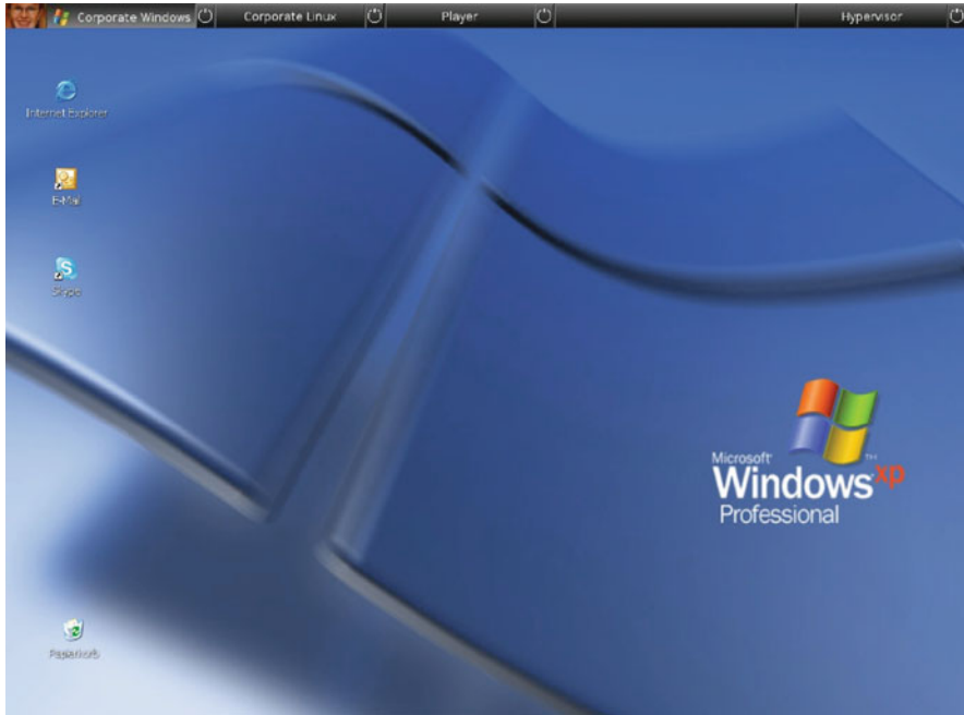
Fig. 9.2 A possible future user interface. The figure shows a novel taskbar, with a sealed image as a means of protection against mimicry by malicious code. The image is only displayed if the hypervisor provided correct measurements. The taskbar also shows buttons for a corporate Windows (running), and buttons for switching to Linux, to a player, or to the hypervisor management interface. Note that the proposed amendment to the user interface requires only little screen space, so that the user interface available for normal work is hardly changed. On wide screens, the novel taskbar could be moved to a narrow side; it could even be hidden if not in uses
