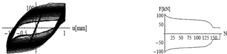
Fig. 11. Hysteresis loop diagram and force - number of cycles diagram, for cycle loading at constant displacement range \pm 1 mm.
