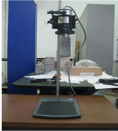
Fig. 3. The Green Luserna Granite specimen connected to the ultrasonic horn. The ultrasonic apparatus (Bandelin HD 2200) consists of a generator that converts electrical energy to 20 kHz ultrasound, and of a transducer that switches this energy into mechanical longitudinal vibration of the same frequency
