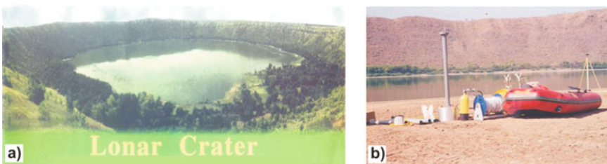
Figure 7.56 (a) The magnificent Lonar Lake. (b) Mini boat and 1.2 m pneumatic Mackereth sampler for recovering under water sedimentary cores from the Lonar Lake.
