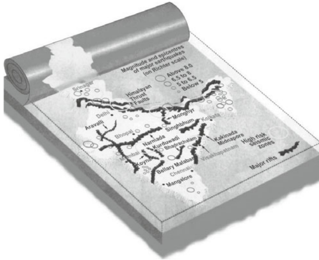
Figure 6.52. Generalized schematic map of major rift zones of Indian subcontinent and their association with seismic activity. The seismicity in peninsular India is found mostly restricted mainly along NE-SW and NNW-SSE trending faults and fractures.
