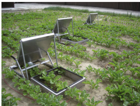
Measurement of N 2 O and CO 2 fluxes with automatic chambers in a sugar beet plot, Estrees-Mons, June 2008 bessou©INRA
