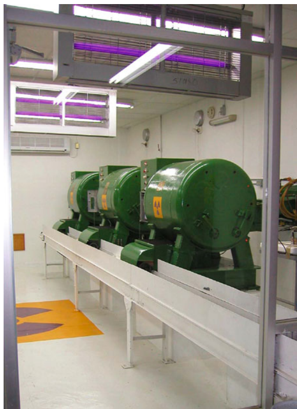
Fig. 4 The three ^{137}\text{Ce} Husman gamma irradiators at the New World screwworm mass-rearing facility in Tuxtla Gutiérrez in Chiapas, Mexico
