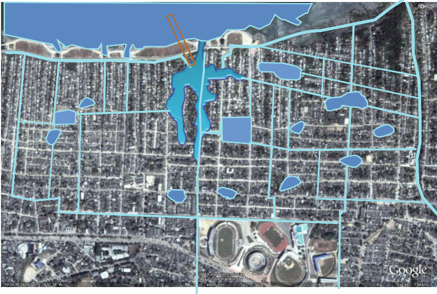
Fig. 4.9 Eco-infrastructure: reuse public space for rainwater storage connected through canals. Source: Compiled by author http://maps.google.com/maps?t=h&hl=en&ie=UTF8&ll=10.411323,-75.495731&spn=0.027098,0.033002&z=15
