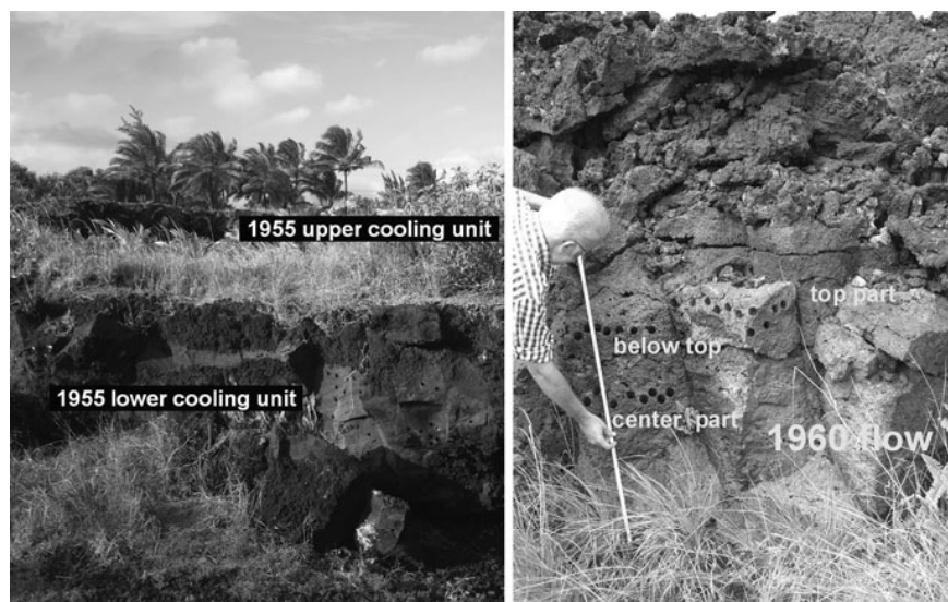
Fig. 14.2 Sampled outcrop of the Kilauea 1955 lava flow, with two cooling units; Kilauea 1960 lava flow cut along the Kapoho-Kumakahi Lighthouse Rd. with drill holes at three levels of the massive part overlain by scoriaceous lava
