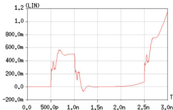
Fig. 1.6 Unstable time domain simulation for non-passive reduced order model of a low pass filter (see also [44])
