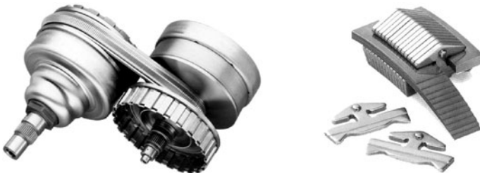
Fig. 1 Pushbelt variator and pushbelt with elements
