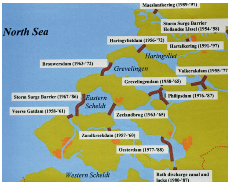
Fig. 83.8 The location, nature and size of the different projects of the Delta works in the Southwestern Netherlands and shows the years when they were completed
