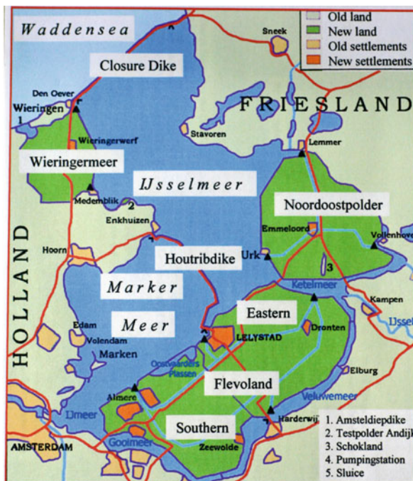
Fig. 83.4 Map shows location, nature and size of the different projects of the Zuiderzee Works in the central north of the Netherlands that were carried out between 1927 and 1975. (Cf. Table 83.1)
