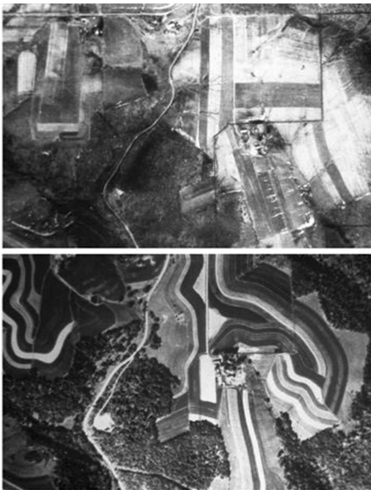
Fig. 77.5 Before and after soil conservation engineering, Coon Creek, Wisconsin. Top: Early 1934. Note rectangular fields and gully systems extending into upland fields. Bottom: 1967. Note contour strip cropping. (Source: Trimble & Lund, 1982)
