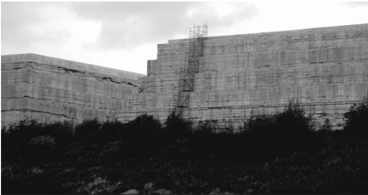
Fig. 27.4 Blocks of sulfur produced during processing, stored at a Syncrude upgrader site north of Fort McMurray, Alberta. No use has yet been found for this a by-product of the upgrading process. (Photograph by the author, June 2006)
