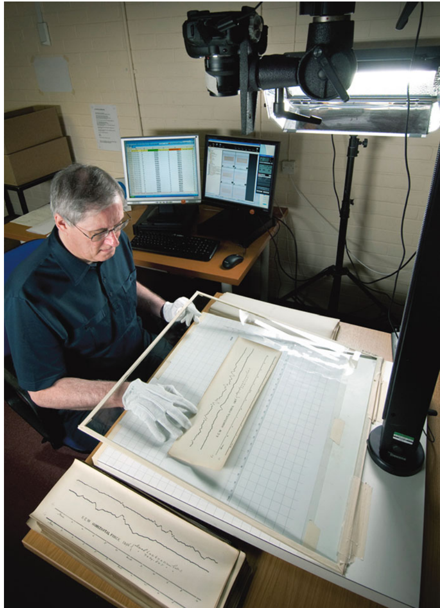
Fig. 7.5 Digital image capture of historical magnetograms. (Copyright: BGS/NERC)
