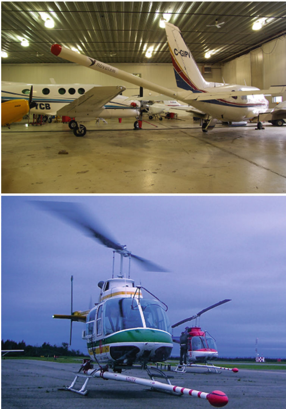
Fig. 4.2 Magnetometer sensor in a stinger ( top ) on a tail of a Piper Navajo aircraft and ( bottom ) on a Bell helicopters (Courtesy of Novatem)
