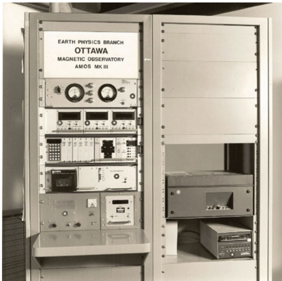
Fig. 5.4 The AMOS Mk 3 is a second-generation automated observatory system deployed at Canadian observatories during the 1980s
