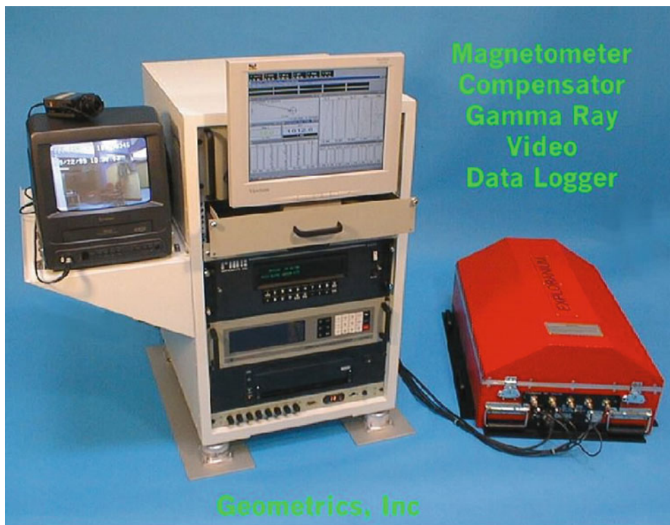
Fig. 4.1 The onboard aircraft data acquisition system mounted on a rack for airborne geophysics (Courtesy of Geometrics)
