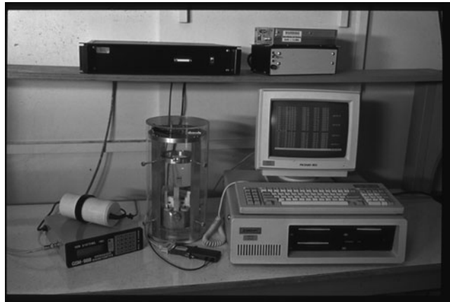
Fig. 5.5 Instruments typical of a modern magnetic observatory. Clockwise from lower right : computer for data storage and system control. Fluxgate sensor in a tilt reducing suspension;
