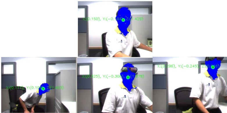
Fig. 3. Some face tracking results where the user wears a pair of stereo glasses. In some cases, the surrounding box of the detected face may include some areas from the background which might have similar color distribution as the face, as shown in
