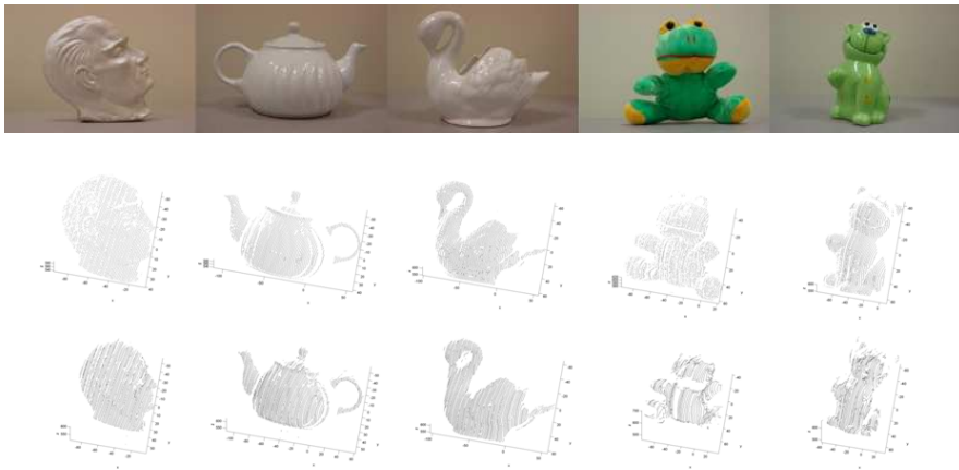
Fig. 1. Point clouds of test objects. Column wise: Atatürk, teapot, dove, soft green frog, green cat. Row wise: Test objects, binary scanner results, ternary scanner results.
