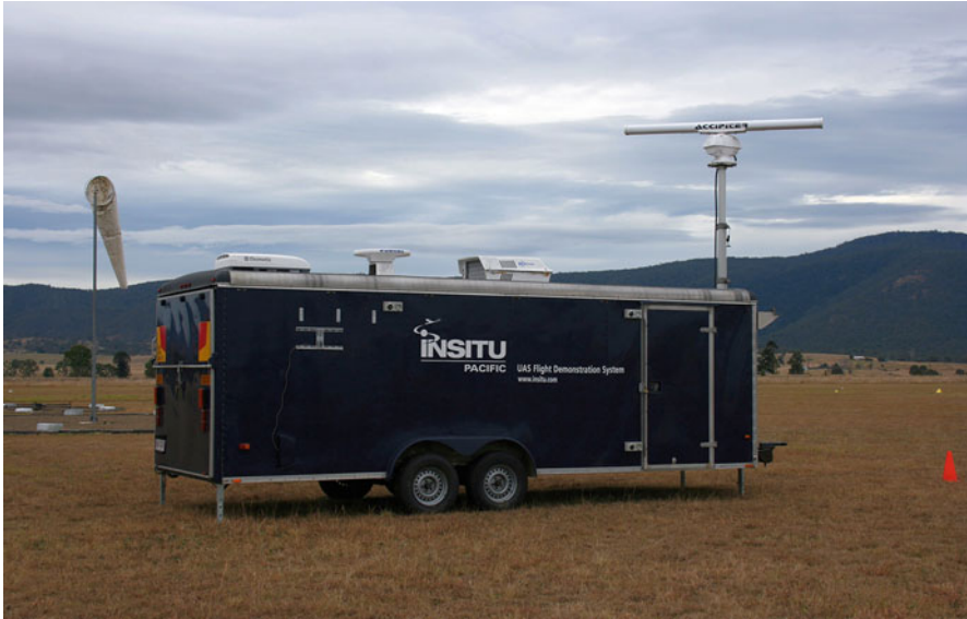
Fig. 92.6 An example mitigation technology: the INSITU Pacific Mobile Aircraft Tracking System with communications, primary radar, and ADS-B In (Wilson 2012) (Image courtesy of Dr Michael Wilson)
