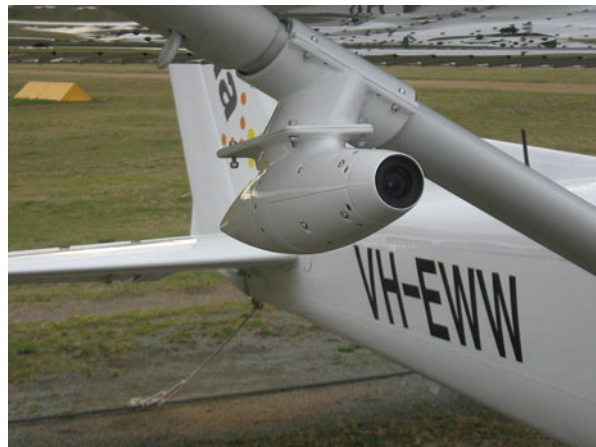
Fig. 92.7 An example mitigation technology: the Australian Research Centre for Aerospace Automation (ARCAA) electro-optical sense-and-act system fitted onto the wing strut of the ARCAA flight test aircraft (Lai et al. 2012) (Image courtesy ARCAA)
