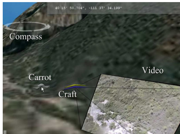
Fig. 99.5 A mixed-reality display fusing control, navigation, and sensor information
