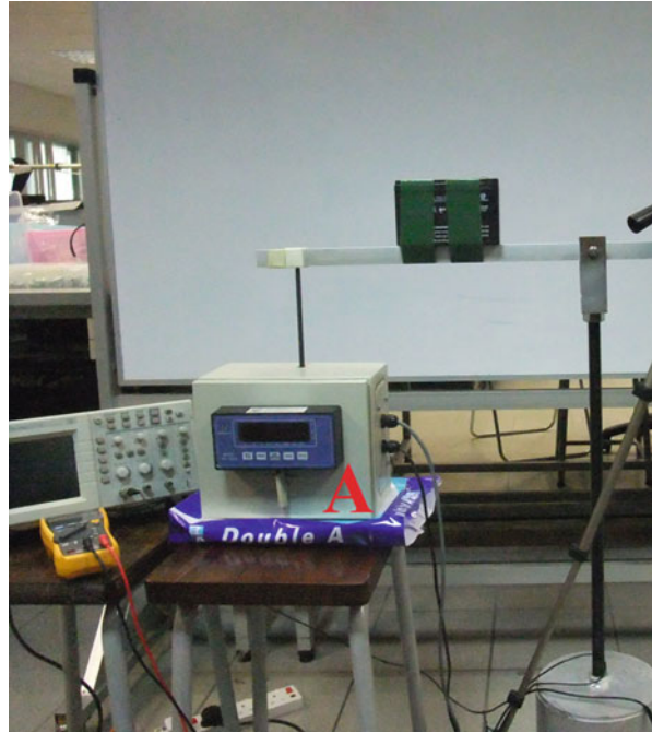
Fig. 49.9 Setup to investigate relation between rotor thrust and rotor rotational speed
