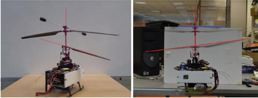
Fig. 49.17 Left : maximum teetering angle of the lower rotor hub; right : maximum flapping angle of the lower rotor
