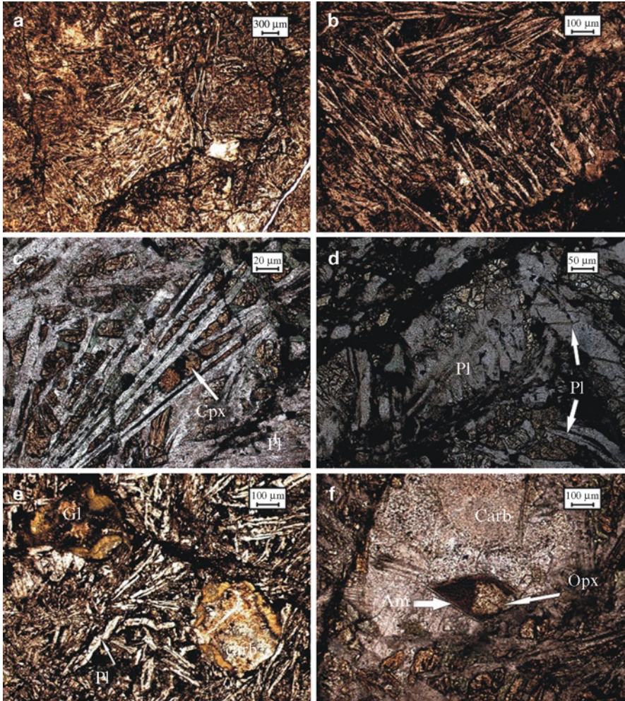
Fig. 13.8 Basalt: (a) Spilite showing variolitic texture. (b) Quenched texture in basalt, containing long, parallel and radiate plagioclase and granular pyroxene (grey). (c) Enlarged view of quenched texture showing hollow core plagioclase filled by granular pyroxene and green glass. (d) Basalt with quenched texture containing curved and dog-tooth plagioclase in contact with hyaloclastite ( top left corner ). (e) Basalt with quenched texture containing hollow core and curved plagioclase and pyroxene in association with clasts of glass and carbonate developed in vesicular cavity. (f) Euhedral brown amphibole (am, kaersutite?) with a core of pyroxene (cpx) in carbonate clast of quenched basalt by late hydrothermal activity. Abbreviation: pl – plagioclase, cpx – clinopyroxene, gl – glass, carb – carbonate, am – amphibole
