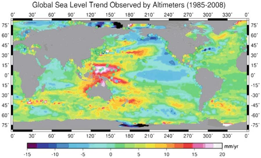
**Fig. 7.7** Sea-level trend observed by individual tide gauges (1900–2006, trend color coded and show as circles) with a global average of  $1.6 \pm 0.4$  mm/year. The background is the satellite altimetry observed short-term (1985–2008) trend of  $2.6 \pm 0.4$  mm/year ( $2.9$  mm/year after GIA effect is corrected), when averaged globally
