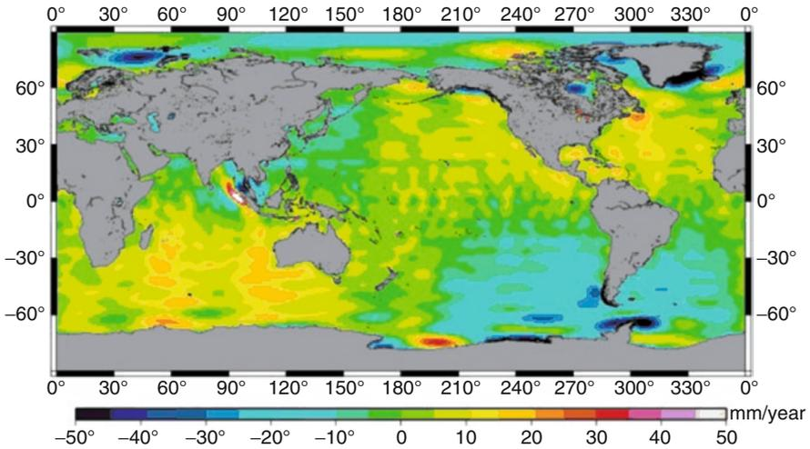
**Fig. 7.9** GRACE observed global ocean bottom pressure interannual variation, 2003–2008 (mm/year). CSR RL04 Level 2 data product used, water thickness change, de-stripping and smoothed at 200 by 300 km by a non-isotropic filter, ICE5G(VM4) GIA geoid and seasonal signals removed, land leakage signal repaired. (Duan et al. 2009; Guo et al. 2010; Guo and Shum 2009)
