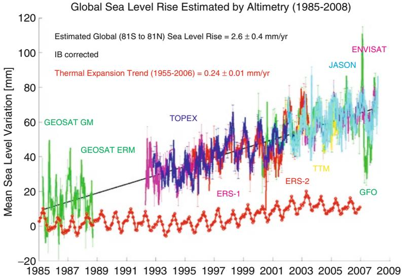
**Fig. 7.6** Multiple-mission satellite radar altimetry (GEOSAT, TOPEX/POSEIDON, ERS-1/-2, JASON-1, ENVISAT and GFO, 1985–2008) observed sea-level trend (2.6 mm/year, 2.9 mm/year when GIA geoid change correction is applied using ICE-5G(VM4) model [Peltier 2004]). There is a data gap between 1989 and 1991
