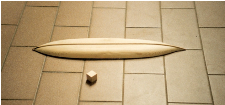
Fig. 2. Evaluation of the volume of the bottom part of the hull of the Syrakosia by weight, model by the author, in scale 1:200.
