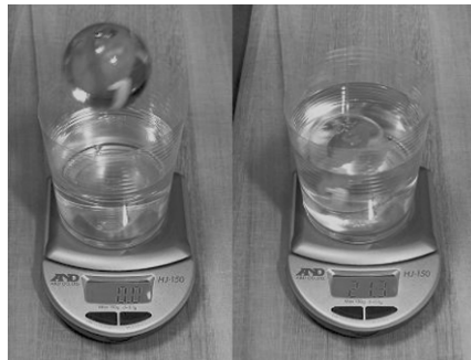
Fig. 6. Glass ball volume measurement.
