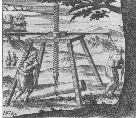
Fig. 9. Spindle hoist by H. Zeising.
