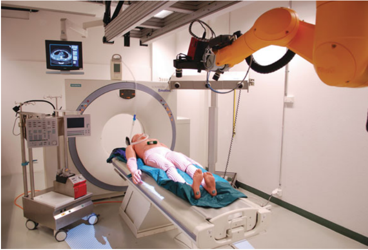
Fig. 9.2.1.1 Right to left: The Virtobot system with mounted surface scanner, optical tracking system for biopsy, CT scanner and heart-lung machine for post-mortem CT angiography
