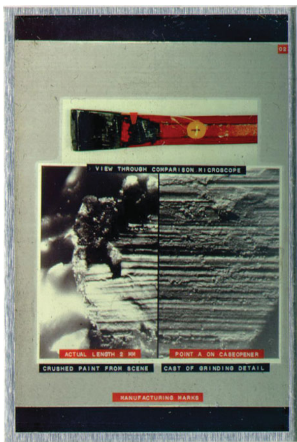
Fig. 7.16.4 Tool mark from the point of entry at the burglary scene. Microscopic comparison used to compare the tool mark in the paint with the tool recovered from the garden at the scene
