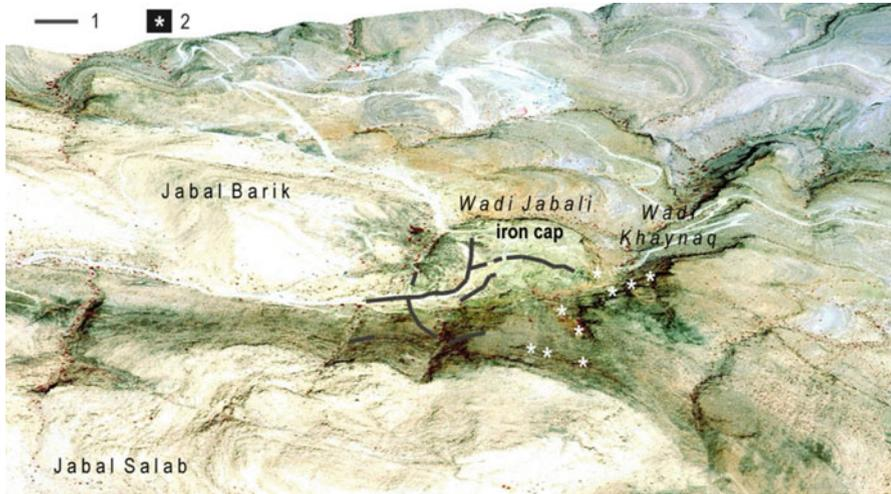
**Fig. 10.5** Detail of the Jabali mine area (3D view). Background: QuickBird data acquired on March 30, 2002. 1 Main canals according to Christmann et al. (1983), 2 main underground mine entries. Note the small watersheds. The shrubs appear as red dots
