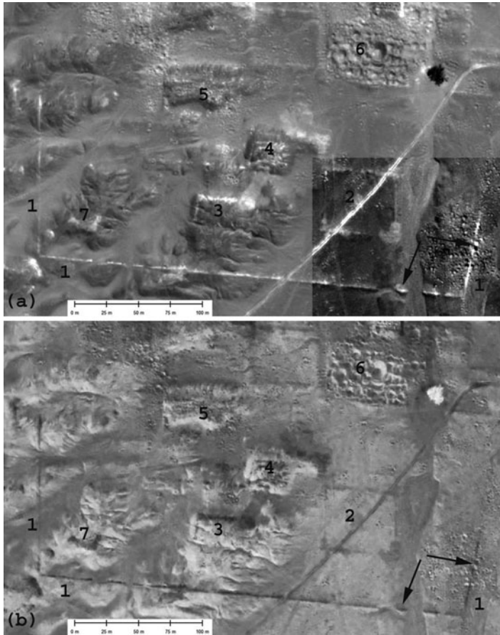
Fig. 14.9 Test site TS1. (a) Panchromatic 2002 QB, in the corner lower right the PC1 result has been overlaid on the panchromatic scene; (b) PC2 result
