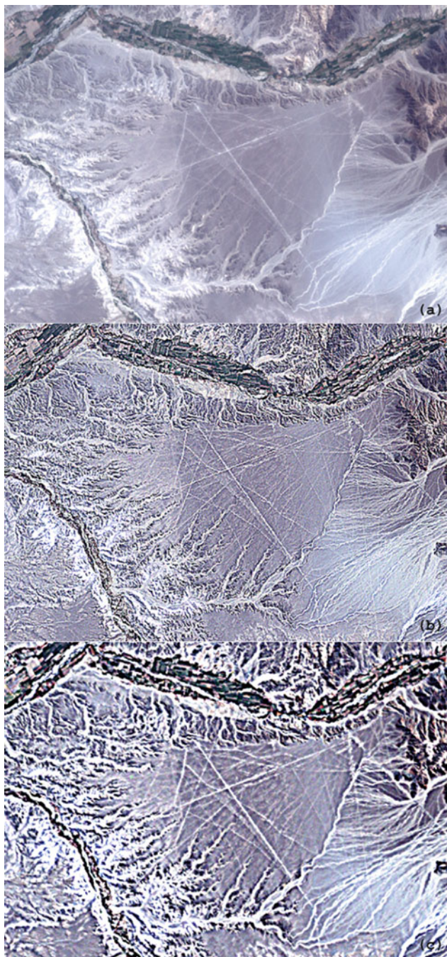
Fig. 2.15 Wavelet transform performed by using open source software IRIS for the same image as in Fig. 2.14
