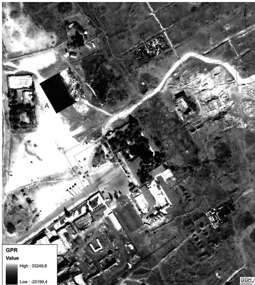
Fig. 6.10 Results of GPR prospecting in central area of Hierapolis, georeferenced on a QuickBird-2 image (processing GGH): (a) the area north-west the Civil Agora; (b) insulae 61 and 70; (c) the area east of the Church with Pillars
