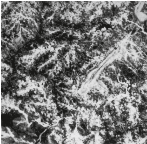
Fig. 4.24 Ratio NDVI image of a part of the area shown in Fig. 4.9. Brighter tones correspond to greater density of vegetation
