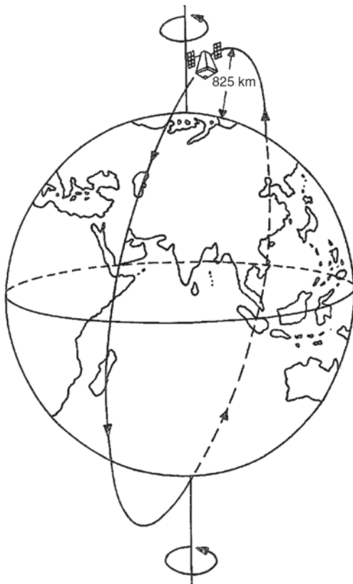
Fig. 4.6 Typical near-polar orbit of an earth observation satellite such as Landsat, IRS etc. As the satellite revolves in N–S orbit, the earth spins from W to E; therefore different parts of the earth are observed by the satellite in different N–S passes
