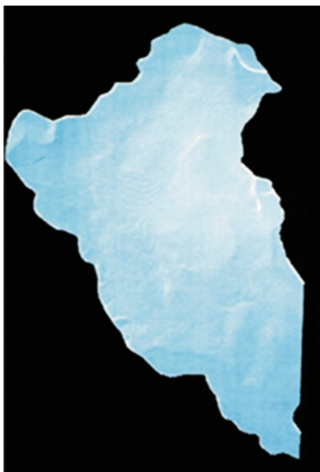
Fig. 6.12 Groundwater table gradient image generated by applying Sobel's filter on Fig. 6.11b. (After Srivastava 1993)
