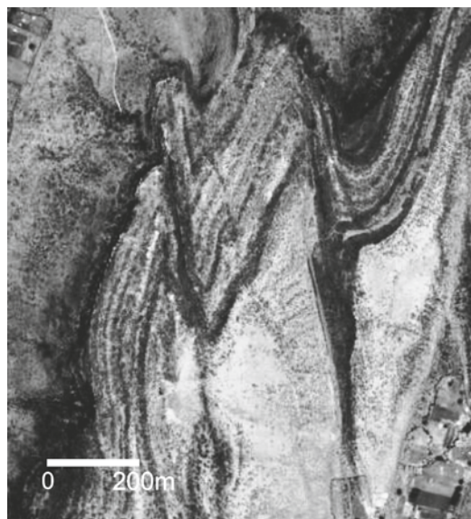
Fig. 2.14 Faults displacing the sedimentary layers of sandstones and shales (Vindhyan Super Group, near Chhattaigarh, India). The terrain has a semi-arid climate. Note the preferential growth of vegetation along fault zones related to the seepage of groundwater. Sedimentary layering is also marked by vegetation banding. Black-and-white image from GoogleEarth
