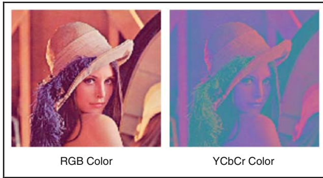
Fig. 20.2 Matlab implementation for rgb2ycbcr
