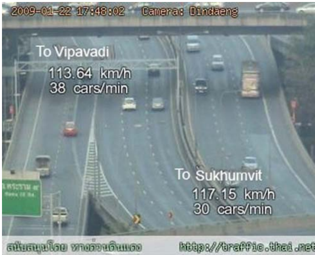
Fig. 21.6 Image classified as light traffic by ANN and as jam traffic by OR technique
