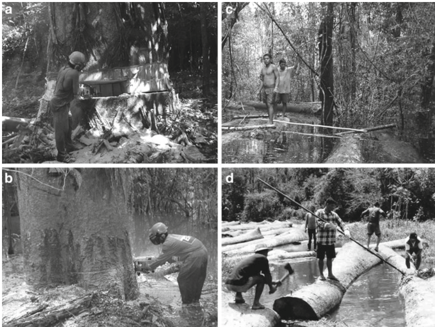
Fig. 20.3 Logging, skidding and transport in the várzea forests. (a) Trees are harvested at the end of the terrestrial phase or (b) when the forests are already flooded. (c) Skidding only can be performed during the aquatic phase. Logs of sinkable high-density trees must be tied between floats of low-density trees ( boiá ) for skidding. (d) Logs are concentrated in lakes or channels and bound together for their transport to sawmills and plywood factories (Photos: PMFC/Mamirauá Institute for Sustainable Development, IDSMD)
