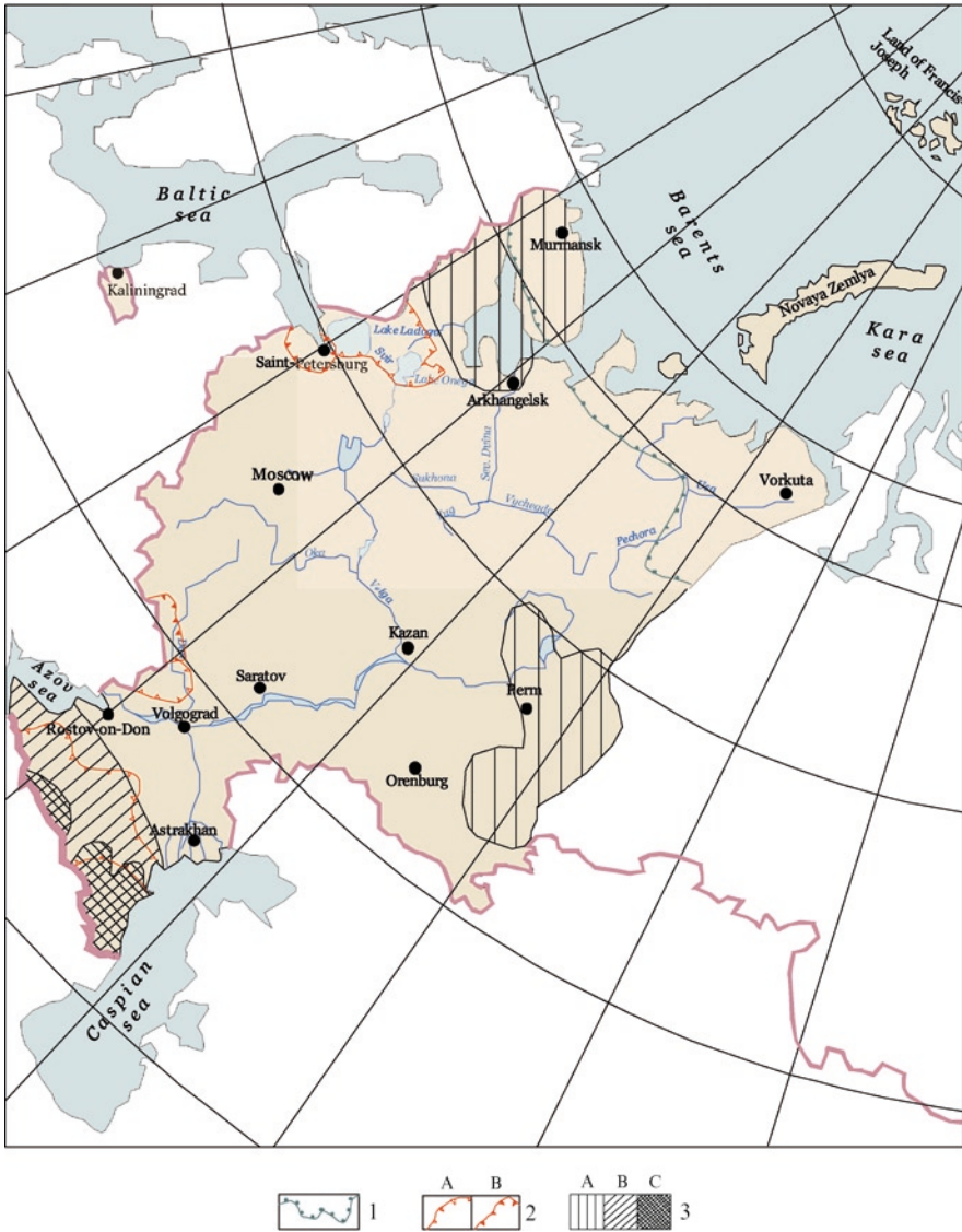
Fig. 2 Locations of endogenous activity zones (seismic risks, volcanism) and increased radon risk. 1 Cryolite zone boundary. 2 Regions of increased (A) and high (B) radon risk. 3 Seismic risk zones: A – with rare random earthquakes with a magnitude up to 4 (according to the Richter Scale); B–C – with constant earthquakes with a magnitude up to 7 (B) and above 7 (C)
