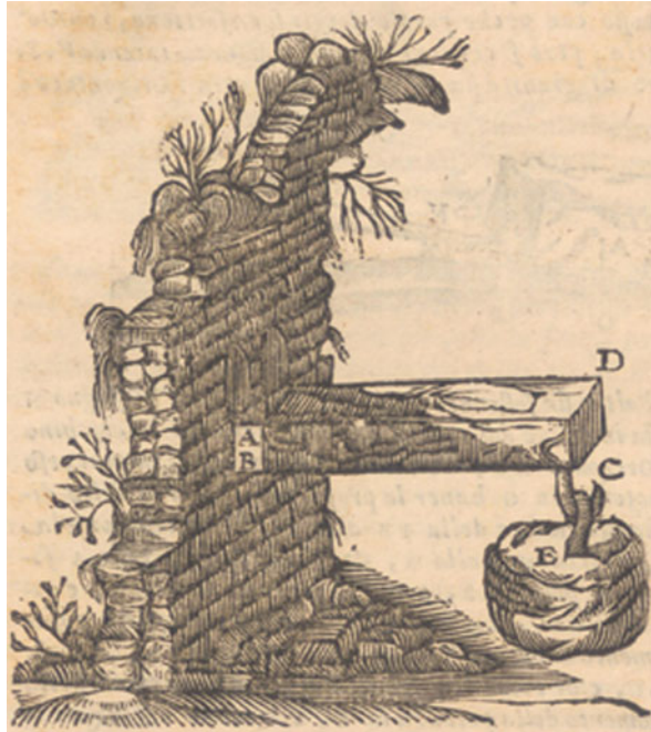
Fig. 4.1 Illustration of Galileo's cantilever model (Galilei 1655, 86)
