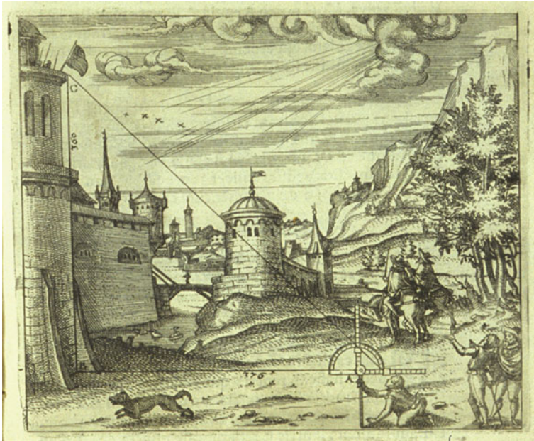
Fig. 2.5 Description of the procedure to measure heights (Zublero 1607b, 19)
