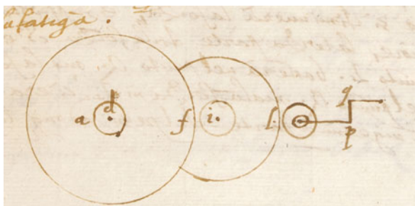
Fig. 3.20 System of axles in the wheels (Galilei 1592–1593a, 30)
