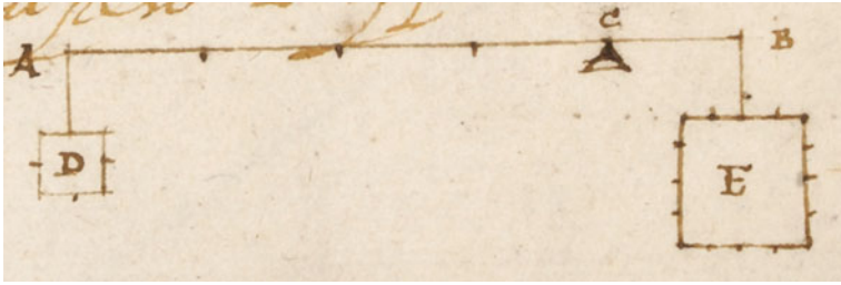
Fig. 3.13 Scale with unequal arms and weights (Galilei 1592–1593a, 15)
