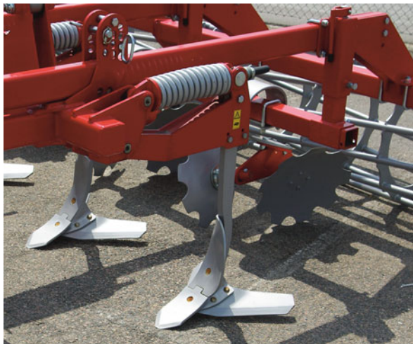
Fig. 11.3 Ducksfoot cultivator (Photo: C. Nilsson)
