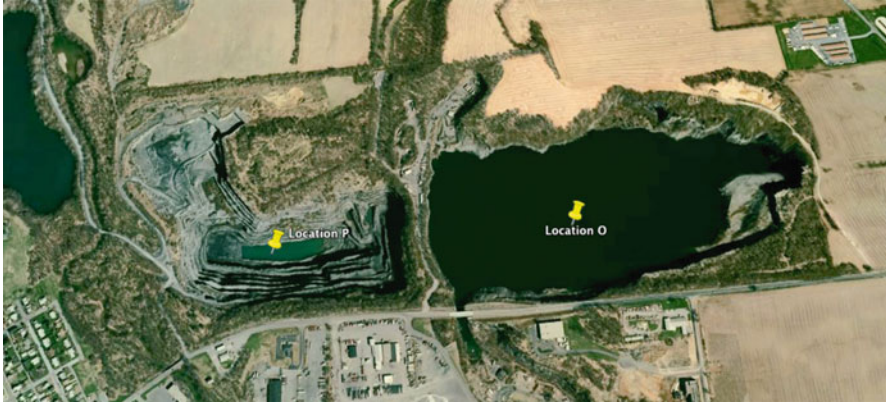
Fig. 13.1 Image from Google Earth displaying locations of an active limestone quarry ( left pushpin) and an abandoned flooded quarry ( right pushpin). The lake level in the abandoned quarry is the local groundwater table; pumping has lowered the groundwater table in the active quarry
