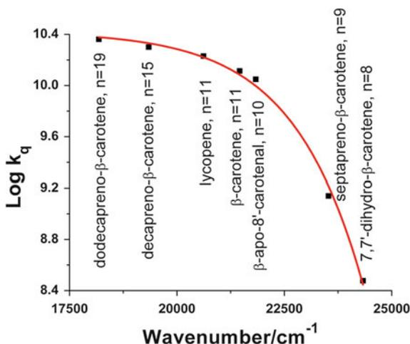
**Fig. 8.2** Graph showing the relationship between the rate constant for  $^1\text{O}_2$  quenching ( $k_q$ ) and the wavenumber of the lowest energy ground state absorption maximum for a range of carotenoids in benzene, adapted from [64]
