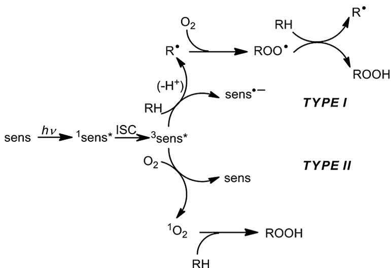
**Fig. 8.1** Reaction scheme for photosensitised oxidation, showing type I and type II initiation
