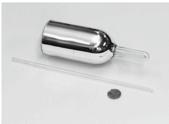
Fig. 14.2 Silvered quartz Dewar and phosphorescence tube for low temperature work. The sample is placed in the narrow tube, which is then inserted into the vertically held liquid nitrogen filled Dewar. Excitation and emission is carried out through the unsilvered nipple on the Dewar. The 5p UK coin, included to give some idea of scale, has a diameter of 18 mm
