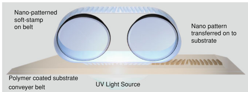
Fig. 13.9 Schematic of roll-to-roll nanoimprint lithography process
