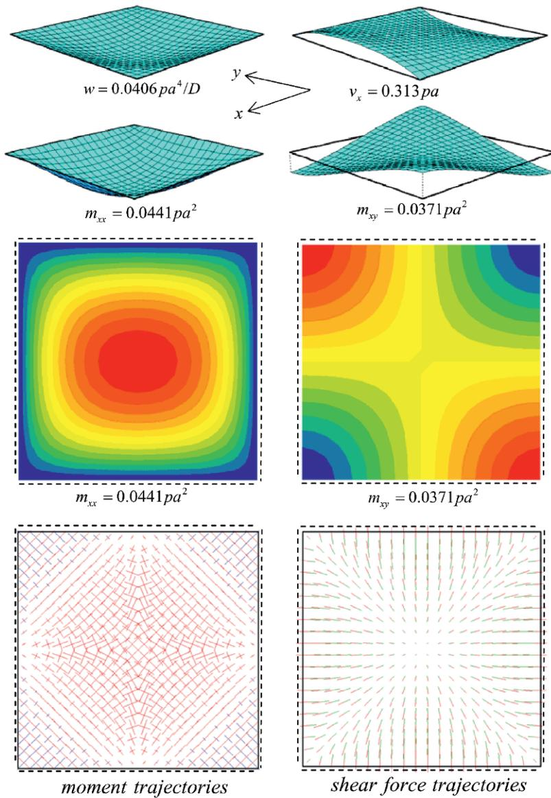
**Figure 13.1** FE results. Square plate. Simply-supported. Distributed load.
