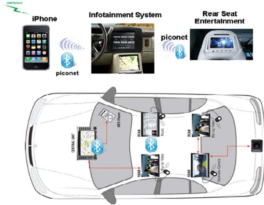
Fig. 2 Pervasive ad hoc vehicle network using bluetooth
