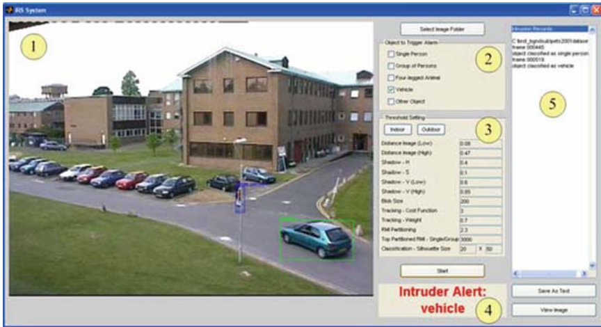
Fig. 9 Screenshot of the user interface program with an intrusion alert, where the numbered items are, as follows: (1) image frame, (2) “Object to Trigger Alarm” panel, (3) “Threshold Setting” panel, (4) intrusion alert, and (5) intrusion records
