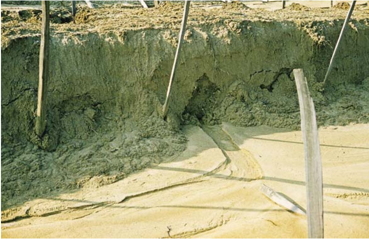
Plate 7.5 Loess degradation through piping. Underground passages formed by impounded water around a vine pole on a terrace surface (top left) in the course of time, conduct water to the lower terrace (centre), Nagy Kopasz Hill, Tokaj (Csorba 1988)
