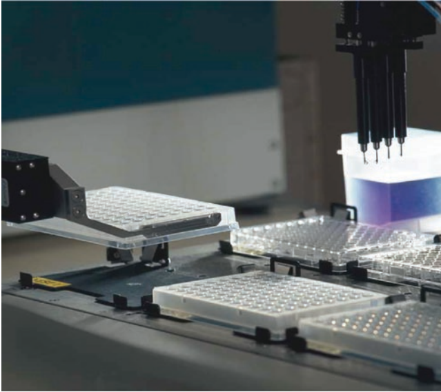
Fig. 6.3 Automation of pipetting procedures is the first obvious moment in regards to improving work conditions and throughput
