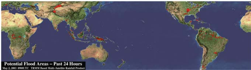
Fig. 1 TRMM rainfall threshold-based flood potential Map : red regions show areas that have received a 24-hour rainfall accumulation (May 2, 2003) > 35 mm
